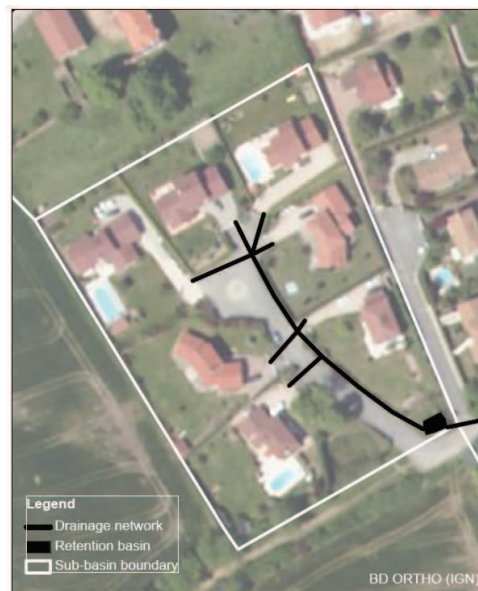
Figure 3: Aerial photograph (BD ORTHO IGN) showing the urban subcatchment delineation following the principle of proximity. This subcatchment is connected to a retention basin.
