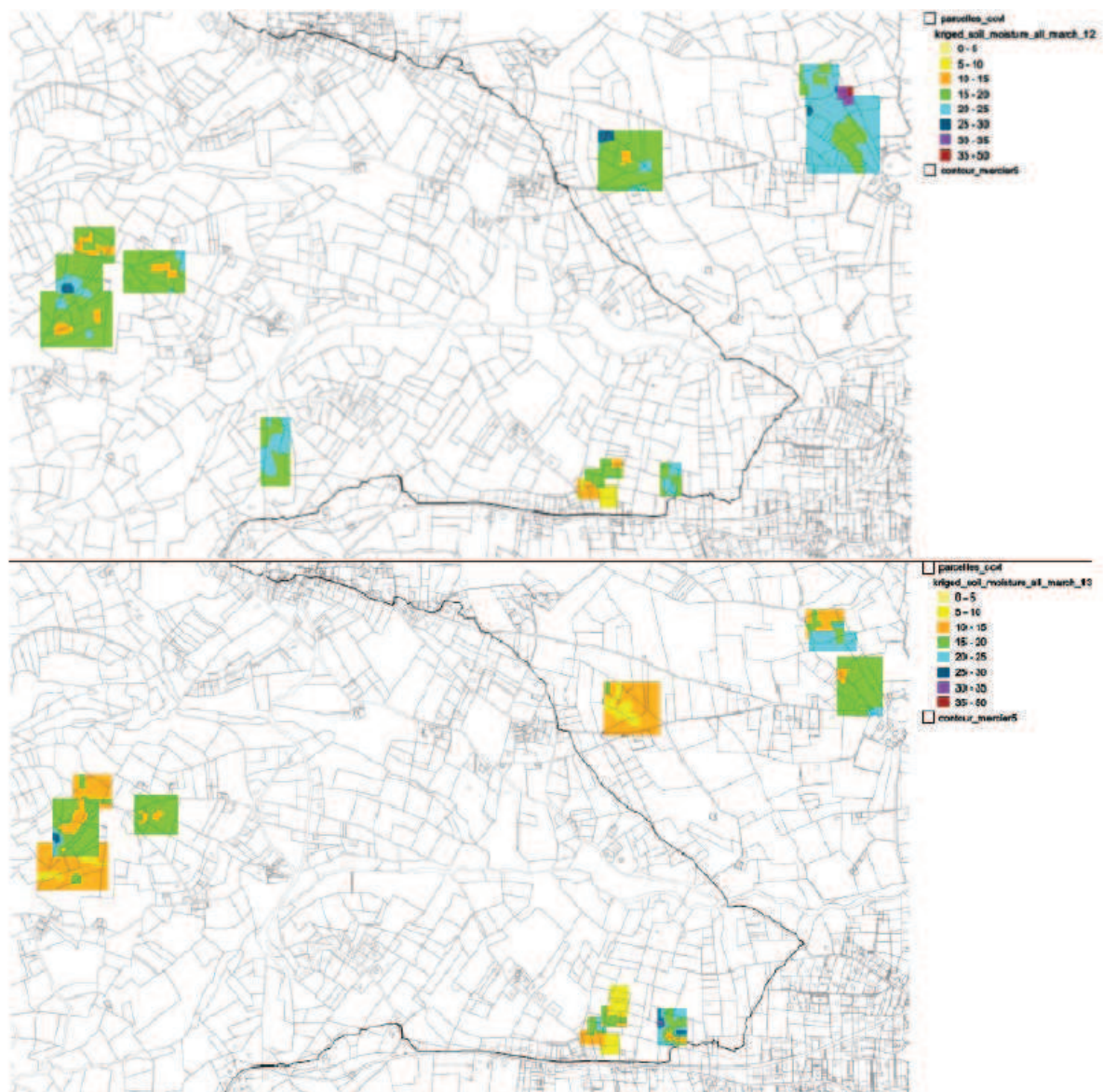
Figure 3.3.4.: By kriging interpolated soil moisture maps of bare soil parcels in the Mercier and Ratier catchments. The data were obtained by TDR measurements along several transects. The upper map is on the 12th of March 2009 and the lower map on the 13th of March 2009 (Braud, 2009).
