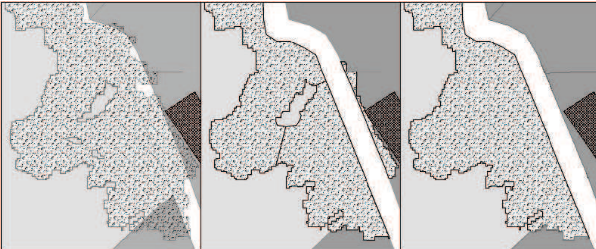
Figure 6.3.2.: Extract of detailed land use map with choice of overlaps (Béal et al., 2009). The original data layers are on the left and the corrected in the middle and on the right. In both cases the connectivity of the road is kept, but in the middle the holes in the wooded area are corrected by creating one hole with the representative surface of all holes and intersection of the polygon with hole. The wooded surface on the other side of the road was unified to create only one polygon. In the right panel, the forest on the other side of the road and the holes were erased, which is less time consuming.
