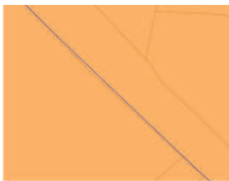
Figure 2: An extract showing the unclean topology of a ditch beside the road. The ditch should follow the road boarder.
