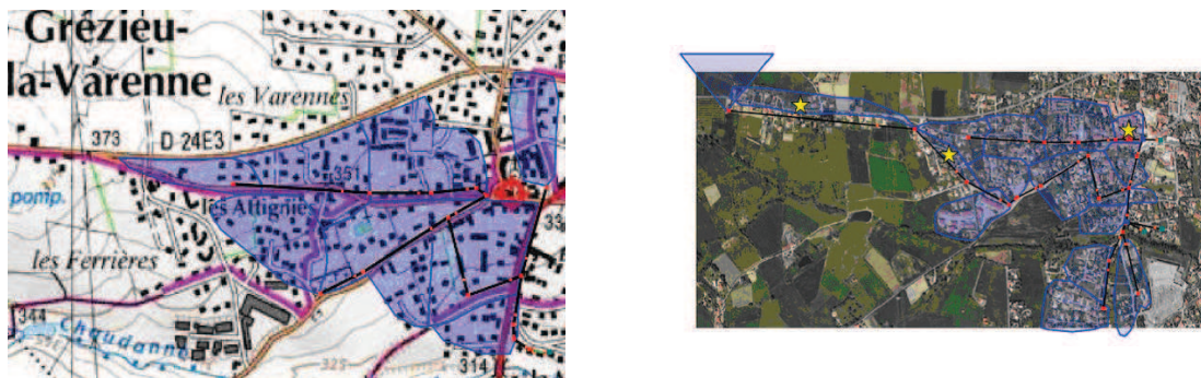
Figure 3.4.7.: CANOE sub-basins and rainwater (up) and combined sewer network (down) for Grézieu-la-Varenne by de la Varde (2010). The rainwater network is connected to the three retention basins at Pont de la Barge.
