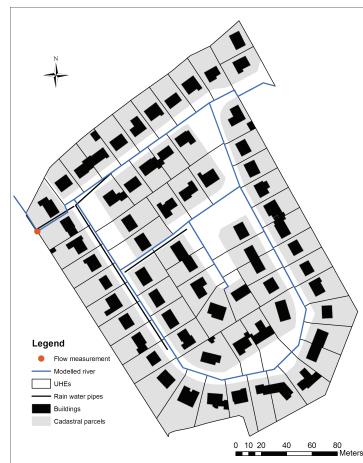
Figure 5.3.5.: The Rezé catchment with its cadastral units, buildings and flow measurement station.
