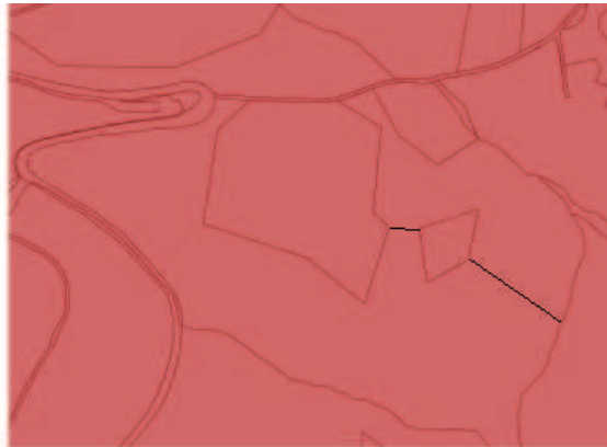
Figure 7: An extract showing a polygon in an another polygon, which creates a hole. A solution of cutting is proposed in black lines.
