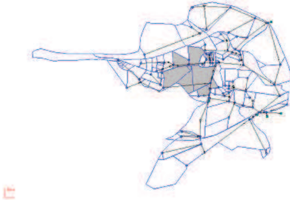
Figure 3.4.2.: Sub-basins and network reaches of combined sewer system at Grézieu-la-Varenne in the Chaudanne catchment for CANOE modelling (Breil and Jouan, 2001).
