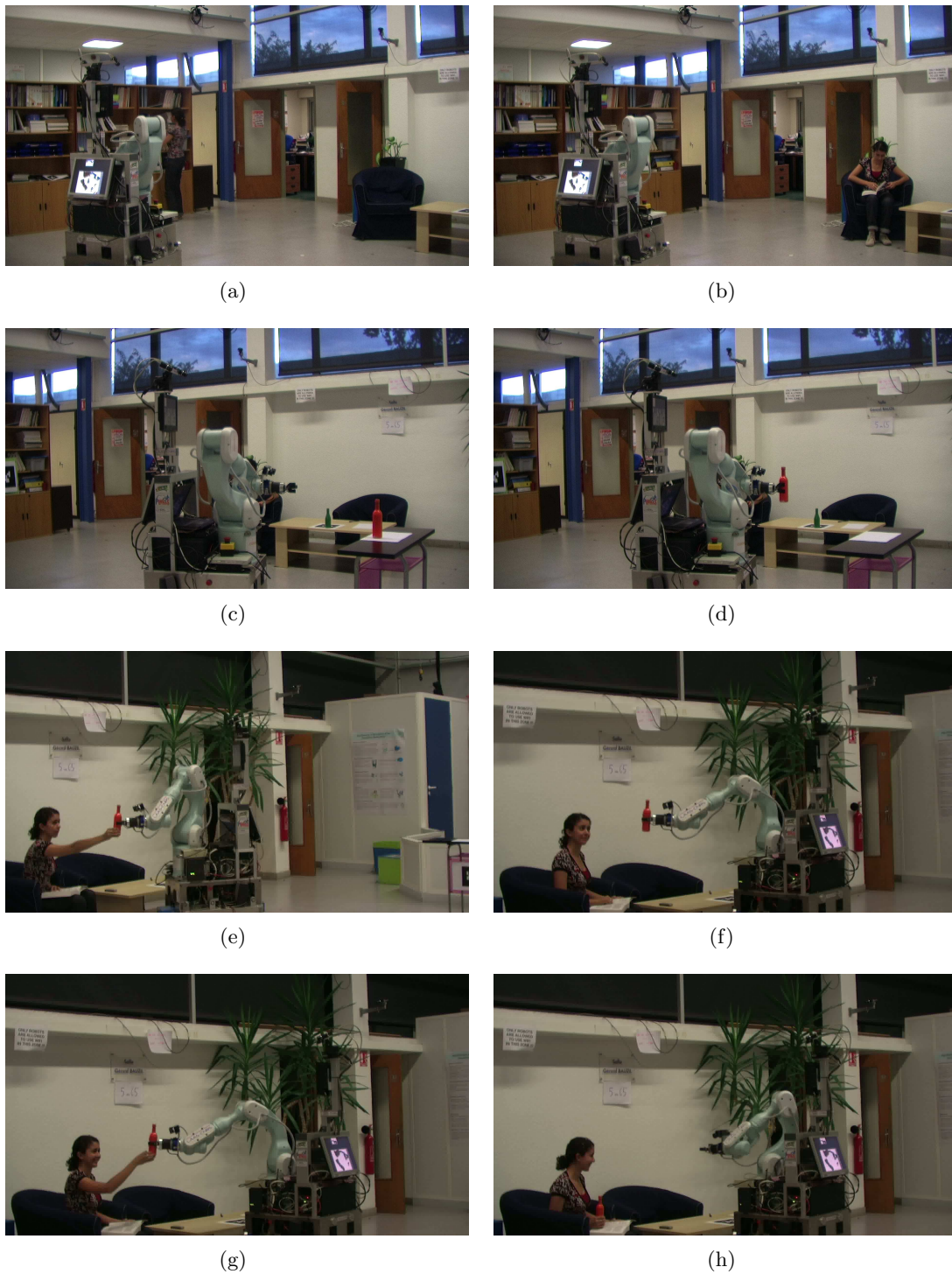
Figure 5.7: Robot recognizing situation and predicting to help and forming a handover joint action
