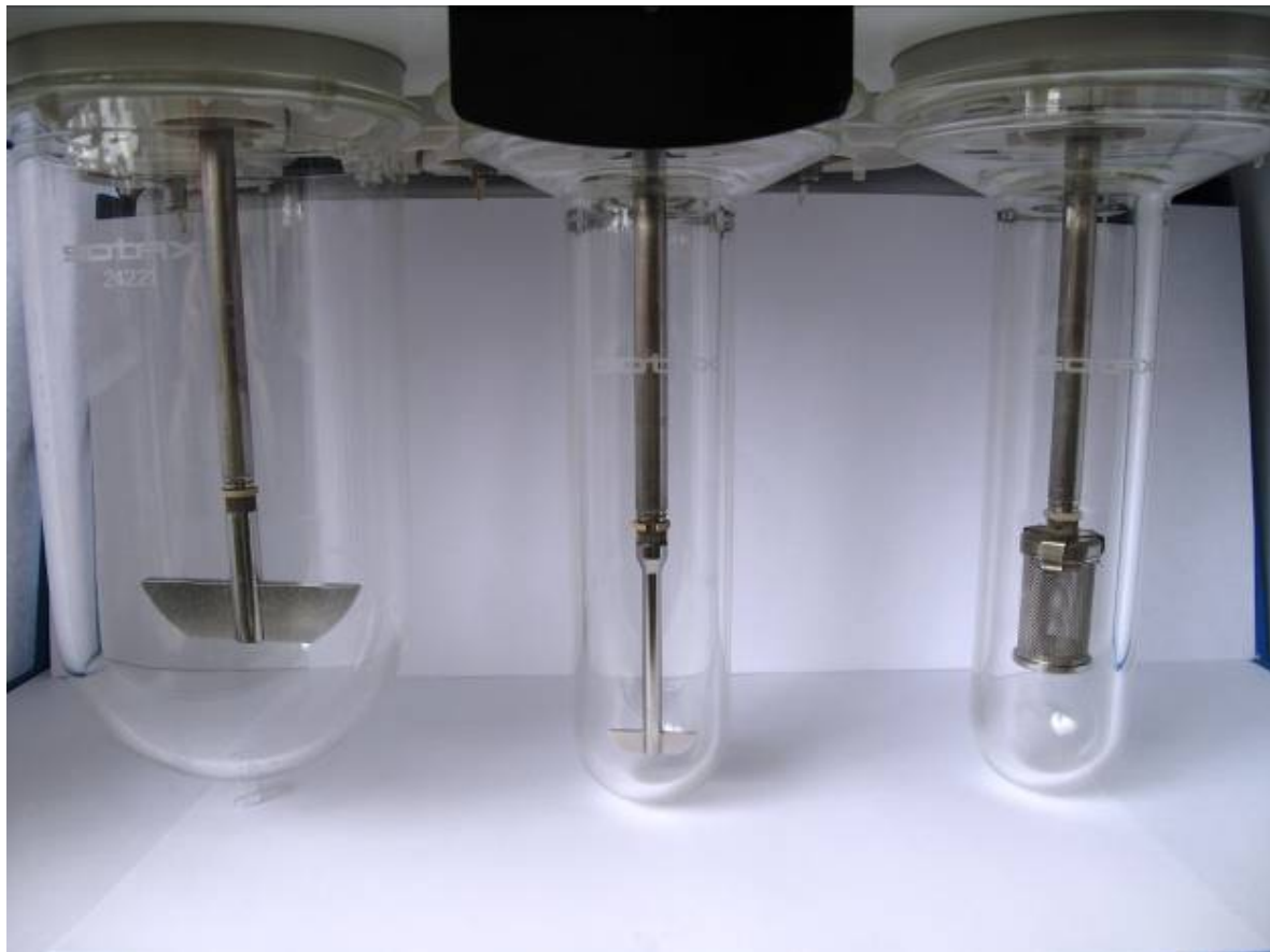
Figure 1 : Small volume vessel setup with small Paddle and Basket. On left side, the compendial one liter vessel with paddle.
