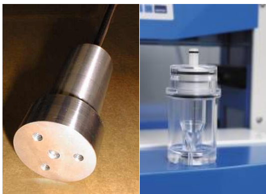
USP <1087> USP<711>, PE 2.9 Figure 3: Apparatus for Intrinsic and apparent dissolution
