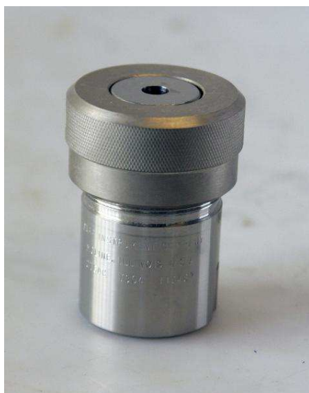
Figure 2-6. Image of a cold-cone seal, Tuttle Roy type (conventional autoclaves).
