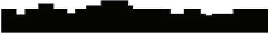
Fig II.6 Schematic representation of a cross sectional cut for a rough surface with a statistical distribution for terrace heights.
