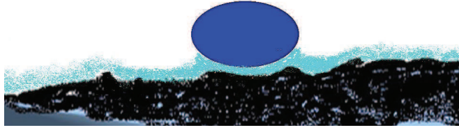
Fig AIV.3 polystyrene particle with radius R in water medium collide with a copper rough surface.
