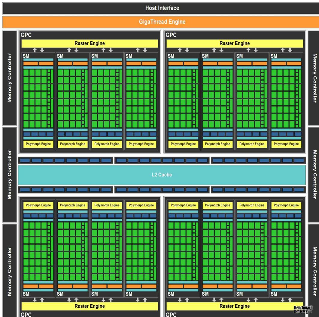
**FIGURE A.11** – Fermi block diagram. The GPU is designed to be highly modular, enabling a variety of different products to be built.
