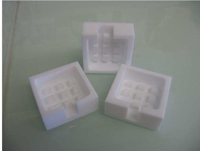
Figure 7.2 Teflon boxes, designed by Philippe Robert, used as support of the slides during coating and rinsing. In this picture one can clearly see the nine small squares on the bottom of the boxes which prevent any contact between the slide and the surface of the box.
