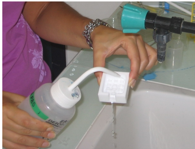
Figure 7.5 Rinsing of a slide inside its teflon box. The rinsing is performed by adding \sim 8 \text{ ml} (volume of the box) of PBS inside the box and then throwing it.
