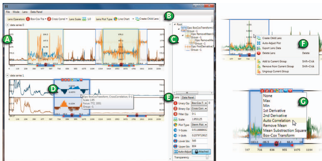
Fig. 1. The ChronoLenses interface includes (A) a charts panel showing the time-series; (B) a lens creation toolbar; (C) a lens analysis pipeline view of (D) the currently selected lens; (E) a property panel showing details of the currently selected lens. A context menu (F) can be invoked to perform lens-based operations, and (G) the lens toolbar allows quick access to a lens' parameters.
