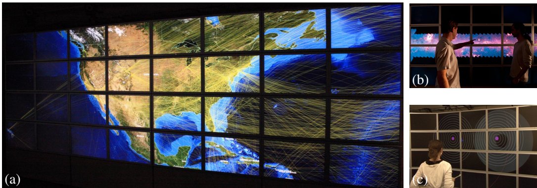
Figure 3.15 : jBricks applications running on the WILD platform. (a) Zoomed-in visualization of the North-American part of the world-wide air traffic network overlaid on NASA’s Blue Marble Next Generation images augmented with country borders ESRI shapefiles. (b) Panning and zooming in Spitzer’s Infrared Milky Way (4.7 gigapixels). (c) Controlled laboratory experiment for the evaluation of mid-air multi-scale navigation techniques (Section 3.1.4).
