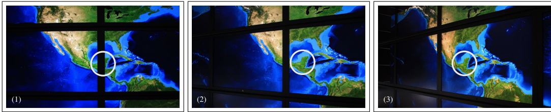
Figure 3.9 : GridScape: the grid formed by monitor bezels on wall displays is often compared to a french window. We designed two interaction techniques that transform that grid into an actual french window. On the map, (1) the Yucatán peninsula (white circle) is partially hidden by bezels. (2) With GridScape, users can reveal that part of the map simply by slanting their body or moving slightly to the right. (3) Moving further right, the entire eastern coast of Mexico can be shown without any bezel occlusion.
