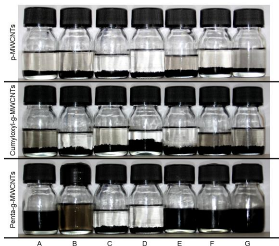
Figure 2-6: Solubility behaviour of pristine carbon nanotubes (p-MWCNTs) after 5 min, cumyloxy grafted CNTs (cumyloxy-g-MWCNTs) after 30 min and pentadecane-grafted MWCNTs (penta-g-MWCNTs) after 2 months in DMF (A); acetone (B); chloroform (C); THF (D); toluene (E); DCB (F); xylene (G).
