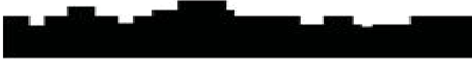
Fig II.6 Schematic representation of a cross sectional cut for a rough surface with a statistical distribution for terrace heights.
