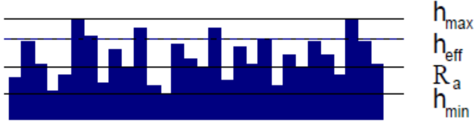
Figure IV.1 (Kunert and Harting 2007). The effective boundary height h_{eff} is found between the deepest valley at h_{min} and the highest peak at h_{max} . For the utilized geometries the average roughness is equal to half the maximum height R_a = h_{max}/2
