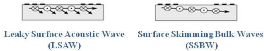
Figure 2.7. Transversal horizontal waves propagated on LiTaO 3 piezoelectric substrate: leaky surface acoustic wave and surface skimming bulk waves.
