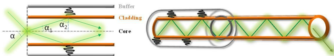
Figure 1.3. Principle of propagation of light in an optical fiber, and optical fiber components with schematic representation of light transmission.
