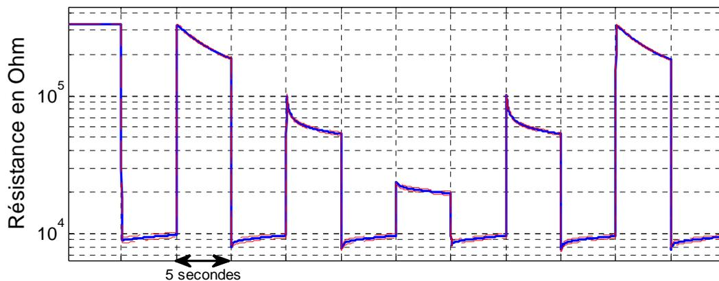
FIGURE 51 : EXEMPLE DE REPNSES TEMPORELLES DU CAPTEUR SnO<sub>2</sub> NANOPARTICULAIRE PILOTE PAR LE PROFIL DYNAMIQUE PRECEDENT (SOUS AIR SYNTHETIQUE)(SUPERPOSITION DES REPNSES SUR 60 CYCLES DU PROFIL)
