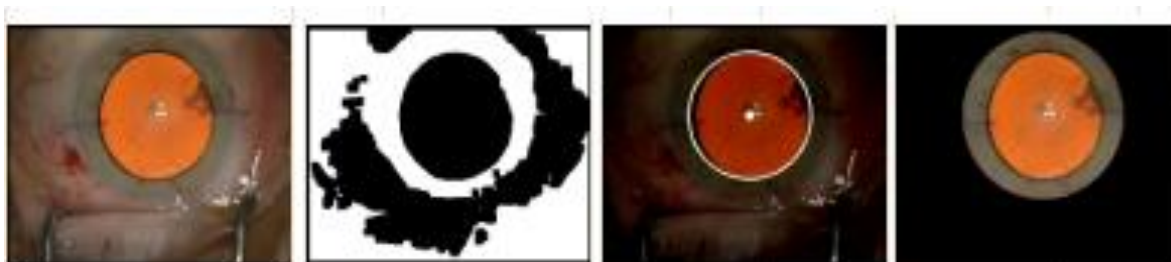
Figure 42 - Different steps of the pupil segmentation. From left to right: input image, 1 st step: creation of the mask, 2 nd step: Hough transform computation, 3 rd step: final segmentation of the pupil.
