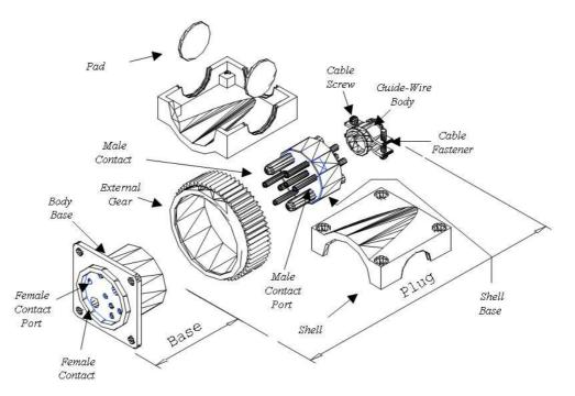
**Figure 8.1 – Electrical Connector**
