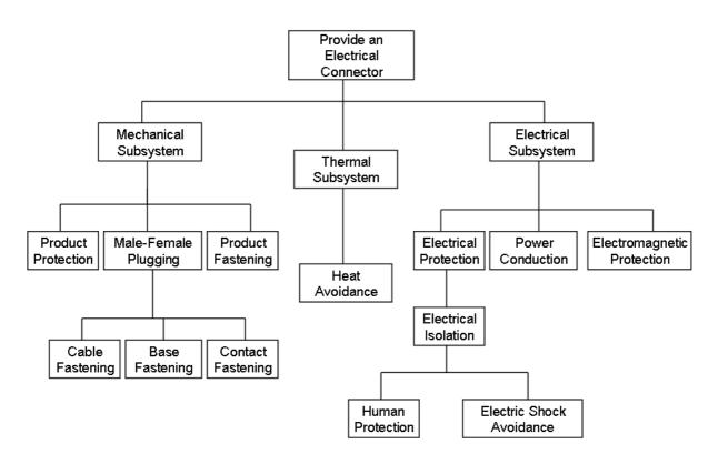
**Figure 8.4 – Connector's Function Model**
