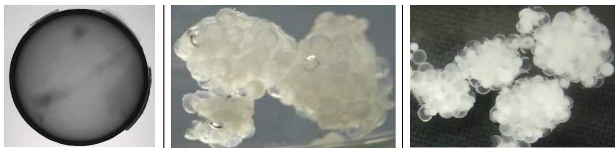
Figure V.13: Picture of a shell, on the left, and pictures of shells agglomerates, obtained during the synthesis of shells with 1% DMPA
