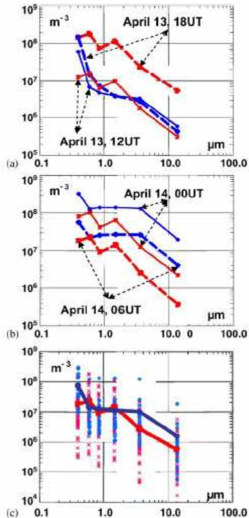
Fig. 7. Number spectra ( $\text{m}^{-3}$ ) of dust particles depositions at Yulin, function of their diameter ( $\mu\text{m}$ ). Red stars: model simulation; Blue diamonds: insitu measurements (MET-ONE). (a) 13 April 2002, (b) 14 April 2002, (c) global comparison between observed and modelled spectra at Yulin during the 11–16 April period.
