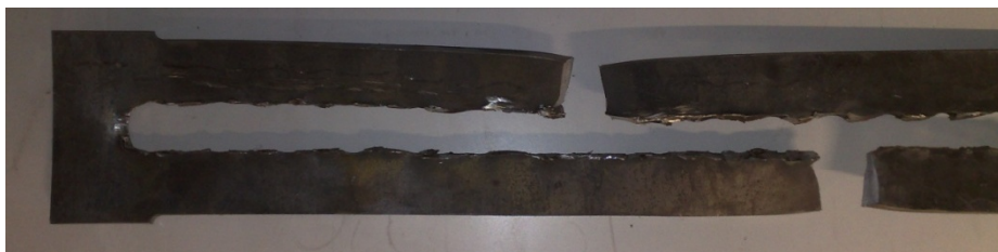
Figure III. 20 : Rupture de la plaque
