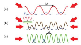
Figure 4.7: Experimental scheme to generate the correlated disorder. (a) Impurities are trapped in a lattice of step 3d. (b) A second lattice of step d is switched on, and the first one turned off. In the final configuration (c), the impurities follow a DRDM distribution. The red arrows symbolize the laser beams of the lattices.
