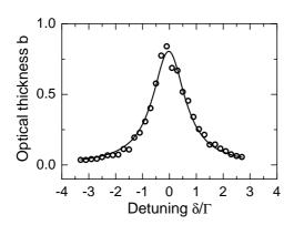
Figure 2.13: Indirect measurement of the imaging probe linewidth. A cloud of resonant optical thickness  $b_0 \simeq 0.8$  is prepared and the optical thickness b is measured vs the laser detuning. The resulting curve is close to a Lorentzian (fitted line) with a width  $\Gamma_m = 1.4 \,\Gamma$ . This broadening is attributed to a laser linewidth of a fraction of  $\Gamma$ , consistent with the diode's specifications (typical value  $\Gamma_L/2\pi = 2$  MHz).
