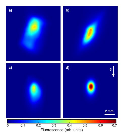
Figure 2.18: Fluorescence pictures of the trapped cloud (a) during the loading of MOT2, (b) after the compressed MOT, (c) after the cloud has been caught in the magnetic trap and (d) after the adiabatic compression. The spatial and color scales remain the same throughout the 4 pictures.
