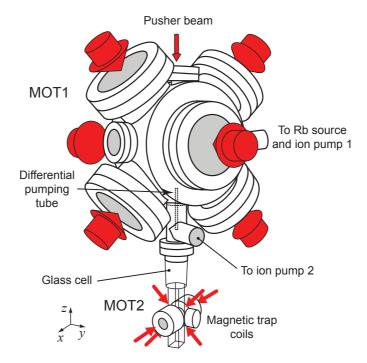
Figure 2.1: Schematic representation of the apparatus with the two magnetooptical trap chambers, the differential pumping tube, and the magnetic trap coils. The red arrows represent collimated laser beams.
