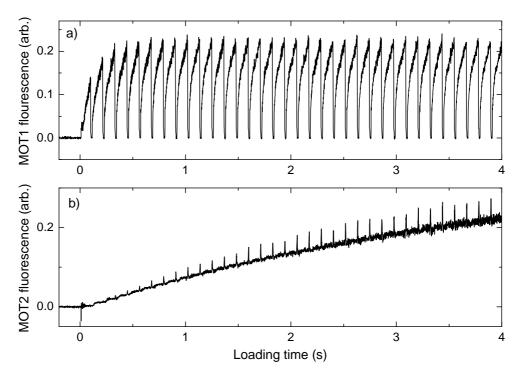
Figure 2.15: Fluorescence signals of (a) MOT1 and (b) MOT2 during the pulsed loading.
