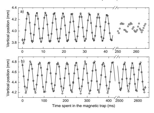
Figure 2.22: Measurement of the trap frequencies. A small magnetic field offset is slowly applied, and abruptly switched off. The cloud position is measured after a variable time of free evolution in the trap plus a constant time of flight (here 27 ms). Vertical trap frequency of (a) the fully compressed trap in which the BEC is produced, (b) a decompressed trap. The lines are exponentially damped sine fits yielding (a)  $\nu_z = 237$  Hz and (b)  $\nu_z = 23.7$  Hz.
