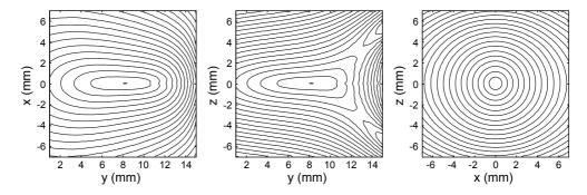
Figure 2.10: Contour plots of the magnetic field magnitude in the IP configuration for a current I=26.7 A (numerical calculation): cut through z=0, x=0 and y=8 mm. Each contour corresponds to an increase of 15 G. The origin (x=0,y=0,z=0) is the quadrupole center.
