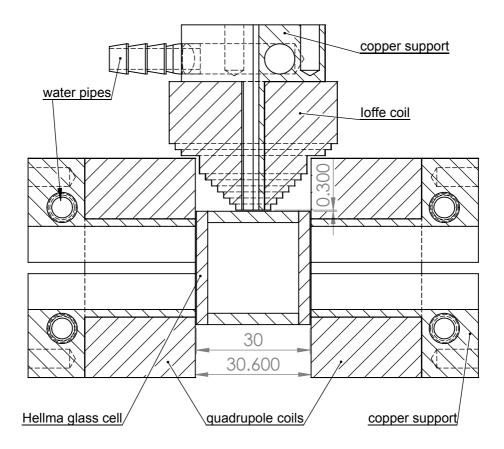
Figure 2.9: Top view of the magnetic trap (cut through the coil centers).
