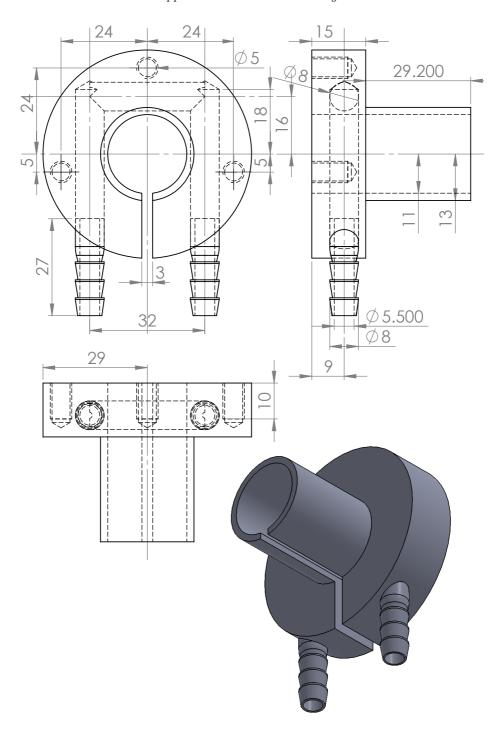
Figure A.3: Quadrupole coil support.
