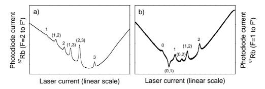
Figure 2.4: Saturated absorption signals used to lock the two lasers. In both cases the six lines corresponding to the three transitions  $F \to F' = F$ ,  $F \to F' = F \pm 1$  and the three crossovers are visible. DFB1 and 2 are respectively locked on the  $F = 2 \to (F' = 2, F' = 3)$  and  $F = 1 \to (F' = 1, F' = 2)$  crossovers of <sup>87</sup>Rb.
