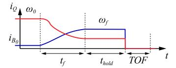
Figure 3.7: A cloud is first prepared in the compressed trap (frequency  $\omega_0$ ), which is then decompressed within a time  $t_f$  by simultaneously decreasing the QUIC current  $i_Q$  and increasing the compensation coils current  $i_{B_0}$  in a controlled way. The cloud then freely evolves in the decompressed trap for a variable amount of time  $t_{\text{hold}}$  before a time of flight measurement is performed (TOF).
