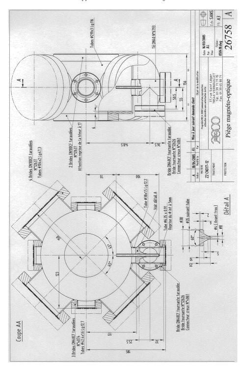
Figure A.1: Main steel chamber.
