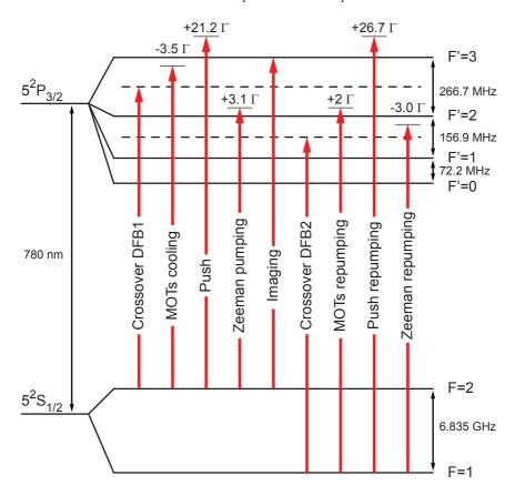
Figure 2.5: Rubidium-87 D<sub>2</sub> line structure and laser frequencies used on the BEC setup. All the frequencies are produced from two DFB diode lasers locked on the indicated crossovers. The detunings with respect to the closest lines (defined as  $\omega_{\text{laser}} - \omega_{\text{line}}$ ) are given in units of the natural linewidth  $\Gamma = 2\pi \times 6.067 \times 10^6 \text{ rad/s}$ .
