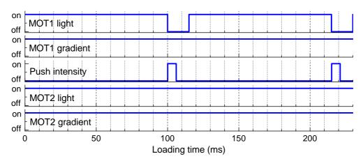
Figure 2.14: Temporal diagram of the pulsed loading of MOT2 from MOT1 (2 periods).
