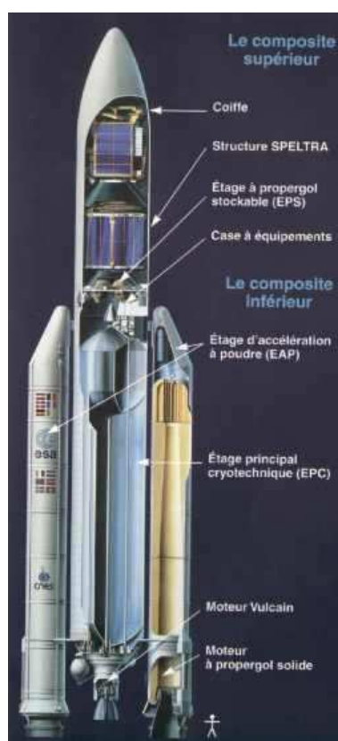
FIG. II.1 – Architecture du lanceur Ariane 5.
