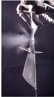
Figure 1.13: Laser peening used in aeronautical applications
