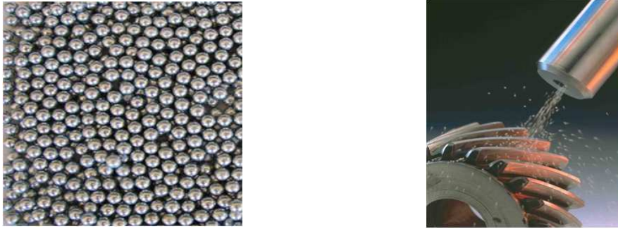
Figure 1.10: Shots (left) bombarding an helicoidal gear (right)
