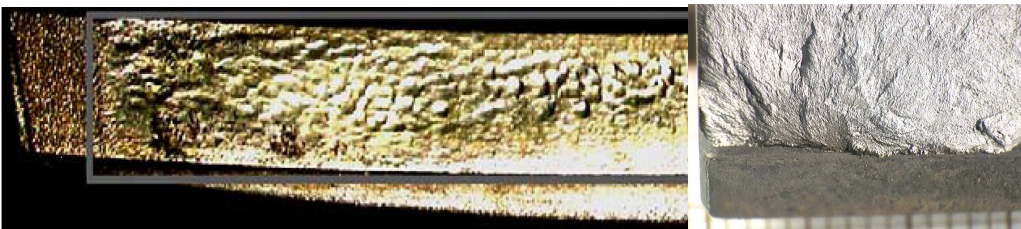
Figure 1.7: Fretting issues observed in blade-roots: wear (left) and fatigue (right)
