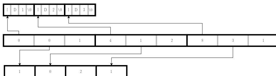
Figure 2.7: Illustration of the adjacency matrix format in MPI_MKDOM2. From top to bottom, arrays represent bytes in: the identifier file, the index file, and the adjacency file. In this example, the matrix stores adjacency relations (ID1, ID2) and (ID2, ID3).
