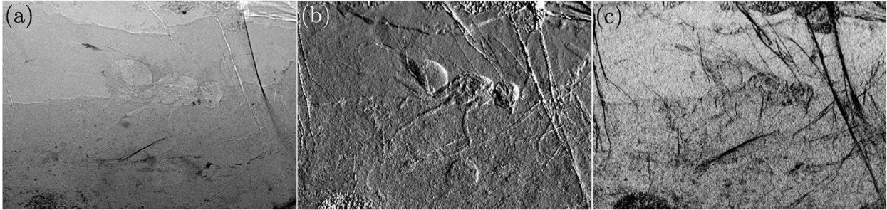
Figure 5.4: (a) Attenuation, (b) differential phase and (c) dark-field (c) projections of the insect in amber obtained during the tomography scan which gave the results shown in Fig. 5.5.
