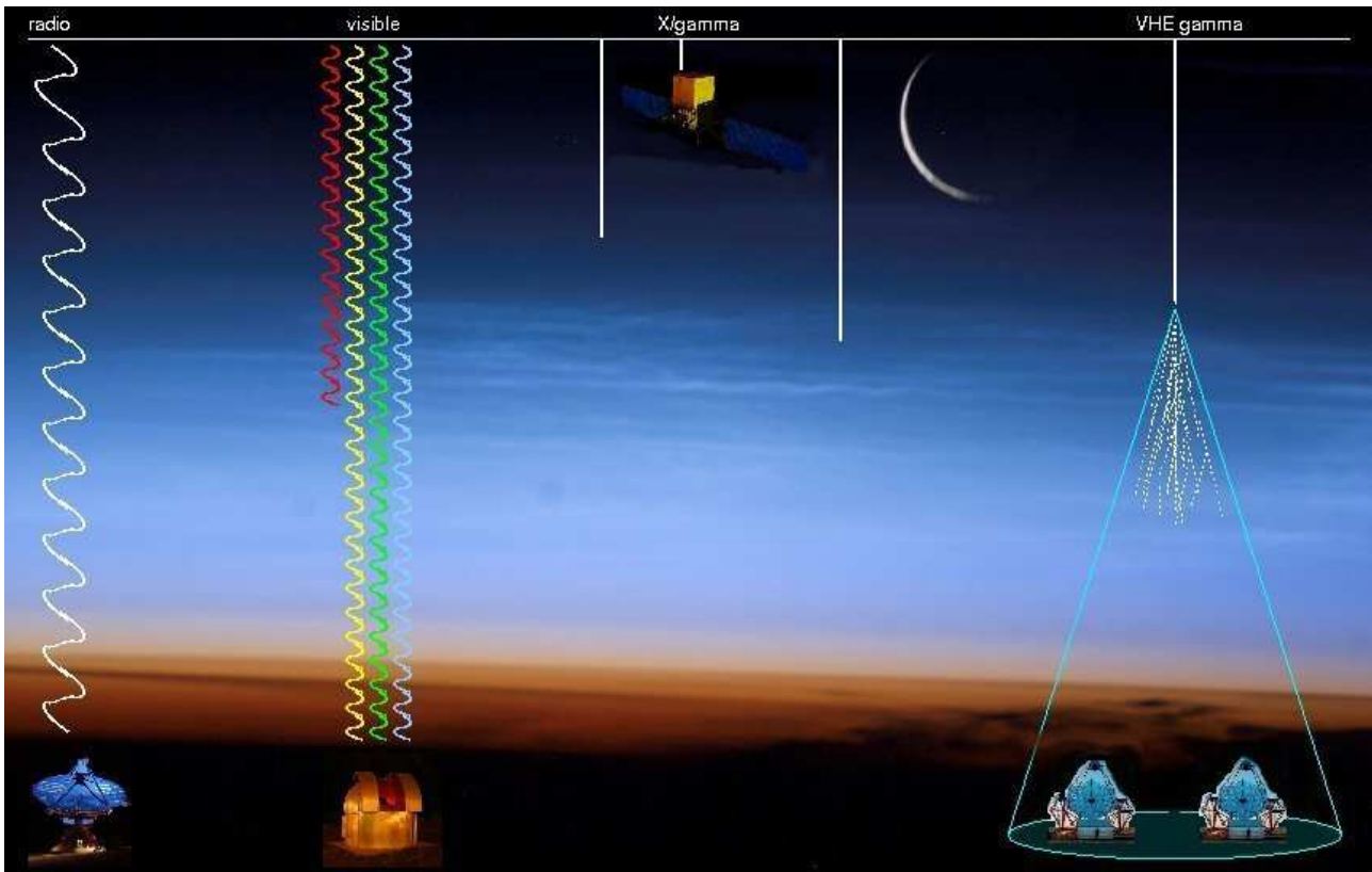
Figure 1.9: Illustration of the link between radiation frequency and the associated instrument. While radio telescopes are only limited by baseline length, and optical telescopes can still be competitive on the ground, higher energy radiation cannot be accessed from the ground until the interaction of the \gamma -ray is energetic enough to generate a detectable Čerenkov flash.
