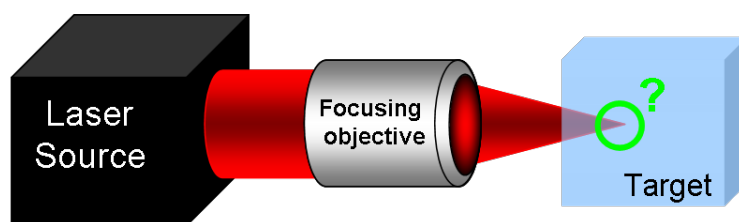
Figure 2.1: General scheme of light focusing of a collimated laser beam.
