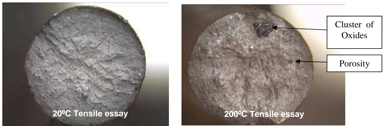
Figure 5.9: Fracture analysis of 0.1% \text{Al}_2\text{O}_3 gamma alumina reinforced alloy
