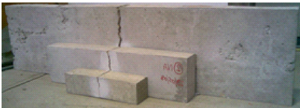
Figure 2.5 Three beams of geometrically similar size in two dimensions (width is constant)
