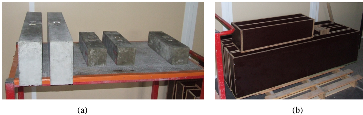
Figure 2.4 (a) Concrete specimens upside down (b) Formwork of concrete beams
