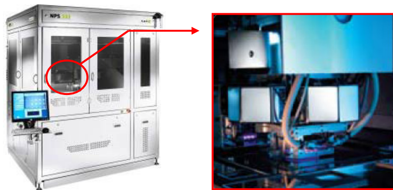
Figure II. 31: a) NPS 300 imprinting tool: overall view (left side) and zoomed view of the imprinting system; b) Schematic illustration of the automated “parallel” demolding step principle (0) and schematic evolution of the separation crack (top view, from 1 to 5).
