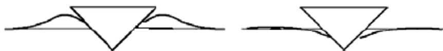
Figure II. 43: Possible profiles that can be met on indented surfaces: left: “pill-up” and right “sink-in”.
