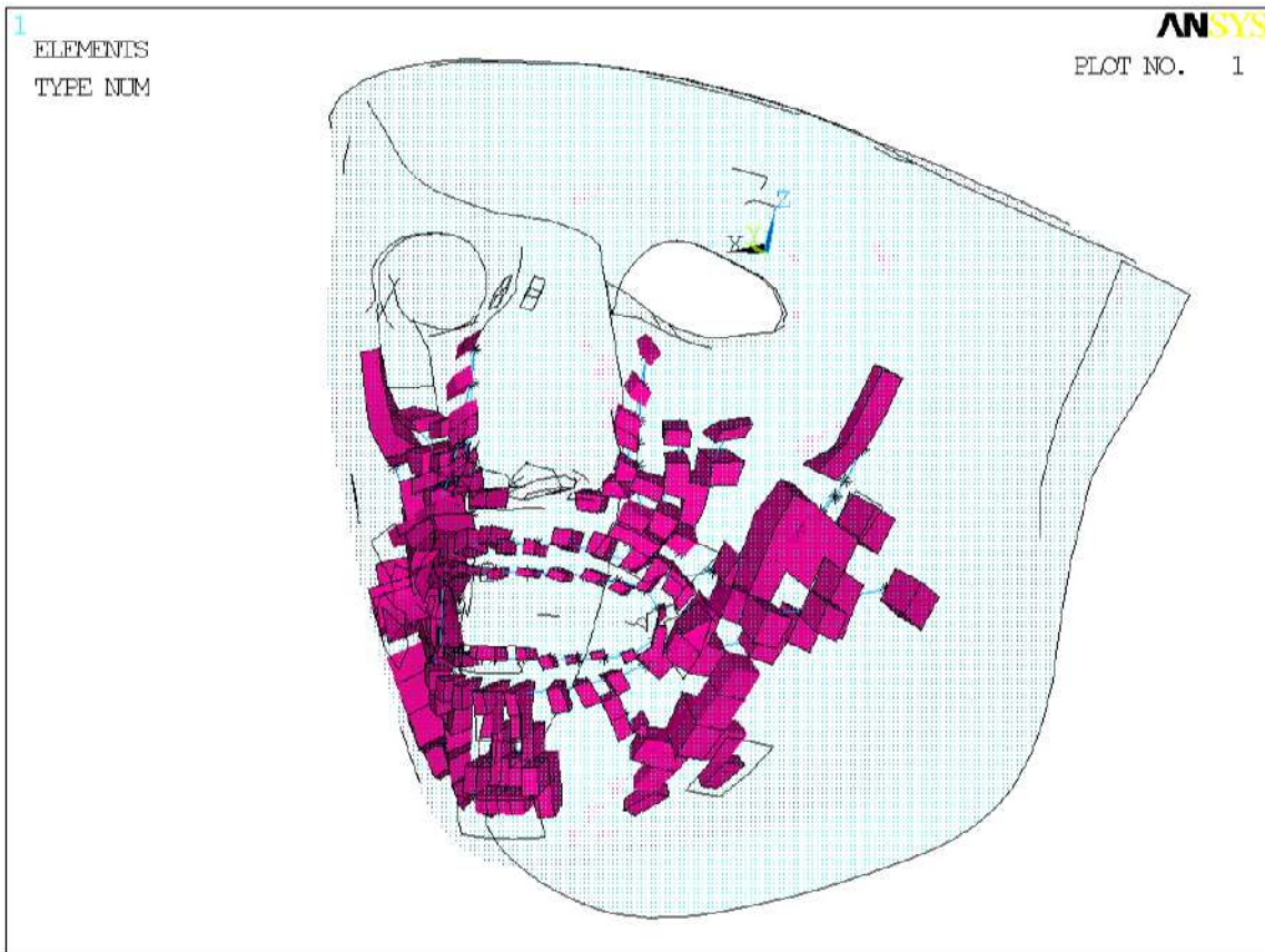
Figure 4.5 Coupling elements between the piece-wise fibres of cable elements and the main mesh.
