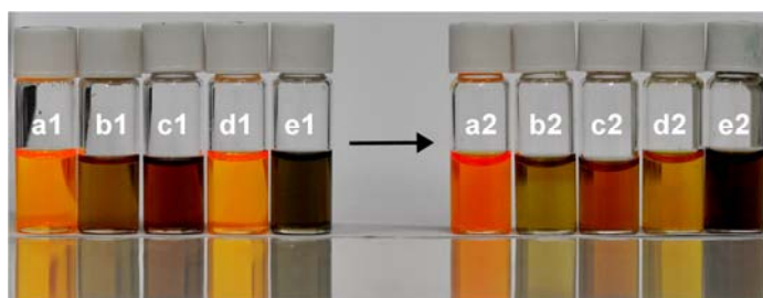
Figure 3.10: Photograph of (a) 6 nm CdSe/CdS/ZnS cores/shell/shell NCs transferred with penicillamine; (b) 7 nm CuInS 2 NCs transferred with MUA; (c) 3.5 x 15 nm CdSe nanorods transferred with cysteine; (d) 4 x 32 nm CdSe/CdS nanorods transferred with penicillamine and (e) CuInSe 2 (edge length 18 nm) triangles transferred with penicillamine. “1” indicates the samples in chloroform and “2” the corresponding samples in water.
