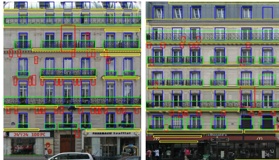
Figure 6.11: Failure cases. Left : the roof windows are not aligned with the facade windows grid. Right : on the top right of the facade a window is over detected. These examples show the typical limitations of our contour and texture based profile projection method.
