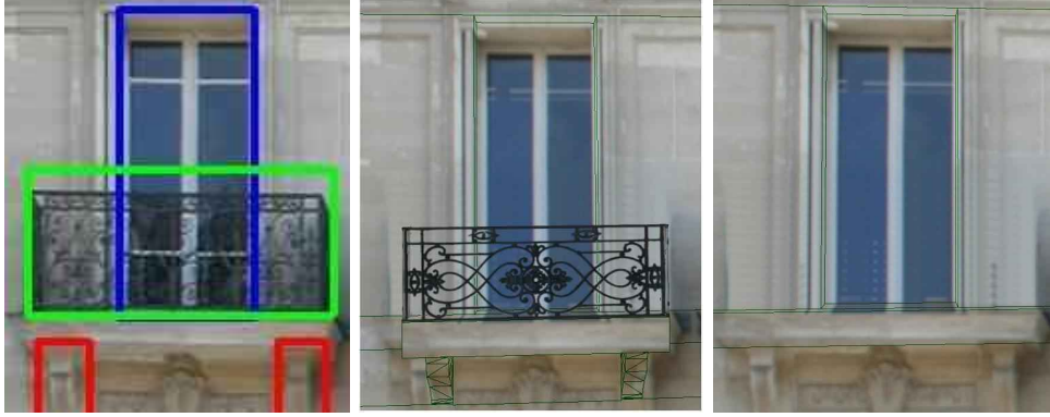
Figure 6.9: Top-down/bottom-up evidence score. From left to right : bottom-up detected elements, top-down candidate structure \theta_1 , top-down candidate \theta_2 . Here likelihood(\theta_1) > likelihood(\theta_2) since the first structure contains a window, a balcony, and two modillions where the second structure contains only a window. The textures are extracted from the same tile in a facade image: the left figure is extracted from the original image where the middle and the right figures are extracted from the inpainted facade image.
