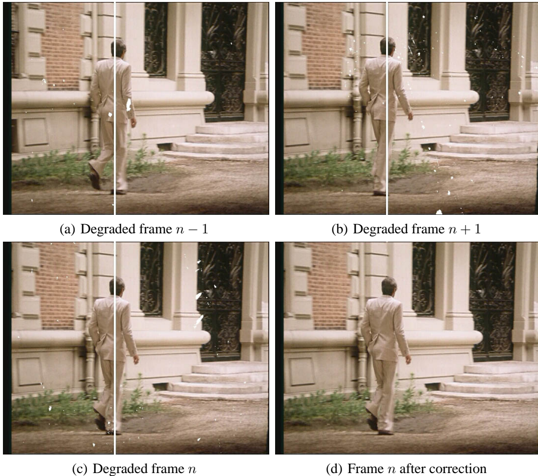
Figure 6.15: restoration of an image sequence with artificial blotches and scratch
