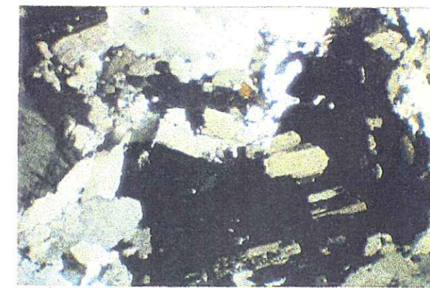
Plate 3.1b Photomicrograph of poikilitic potassium feldspar with ingested, orientated plagioclase feldspar, Ramu granite. (Crossed polarised light)
