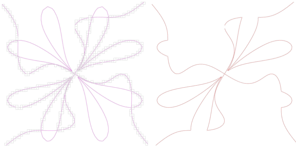
Figure 4.7: Left: defining curves and cell graph. Right: boundary contours of the underlying set.
