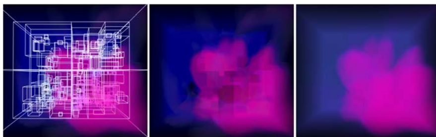
Figure 2.20. Comparison of [KWAH06] of the image quality of slice-based (middle) and GPU-assisted raycasting (right) approaches for rendering a cosmological AMR (Adaptive Mesh Refinement) dataset (left). Artifacts in the slice-based approach are due to insufficient framebuffer precision to correctly blend highly-transparent slices. Source: [KWAH06]
