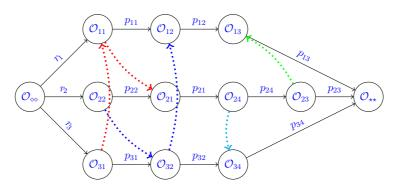
Figure 1.12 – Disjunctive graph representation of solution
