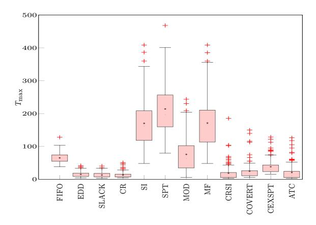
Figure 3.6 – Box plot of  $T_{\text{max}}$  with  $(\tau, \eta) = (8.75, 80\%)$
