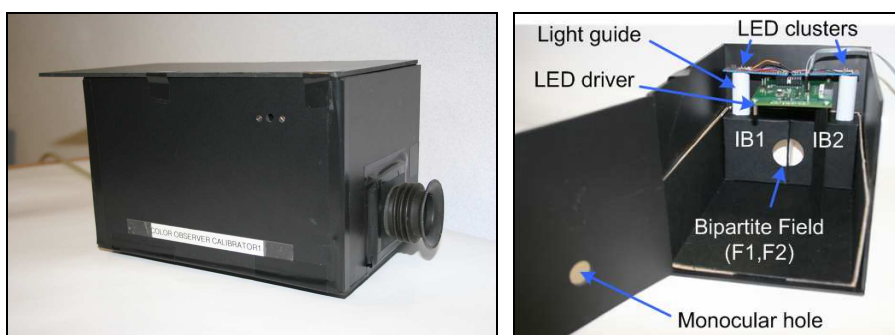
Fig. 6-49. External and internal views of the Observer Calibrator Prototype
