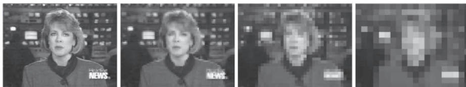
Figure 2.2: Hierarchy of resolution images proposed by (Yang and Huang, 1994). Each square cell consists of n \times n pixels in which intensity of each pixel is replaced by the average intensity of the pixels in that cell. (Courtesy of Yang et al. (2002))
