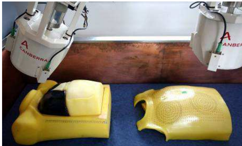
Figure 1.6. The Livermore physical torso phantom with its core chest plates.
