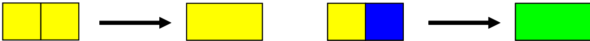
Figure 4.20. Schematic visualization of the rebin functioning when two adjacent voxels with similar (left) and different (right) colors are fused together.
