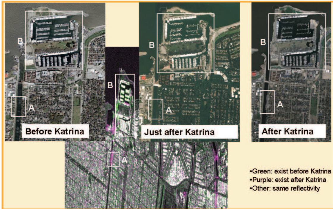
Figure 4.4.8: Change detection analysis by using the SAR reflectivity. Top) three aerial orthophotos taken over the same part of the city before, during and after the Katrina event to illustrate visually the changes due to the hurricane event. Bottom) RGB combination of the mean SAR reflectivity before and after the event, the same as in figure 4.4.7.
