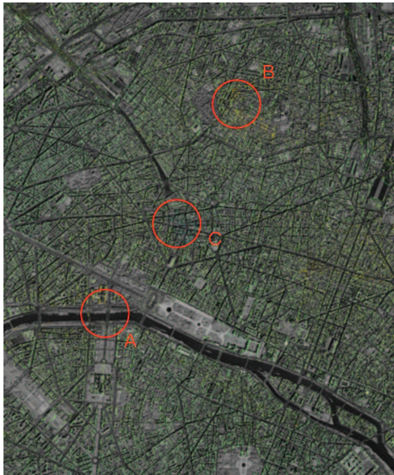
Figure 4.4.15: Linear deformation rate as result of the classical SPN processing for the center of Paris. The covered time period is from 1992 up to 2008, and based in the analysis of about 120 ERS1/2 ad ENVISAT SLCs. The main areas affected by deformation are identified by the red circles. Copyright SPOTIMAGE for the background image.
