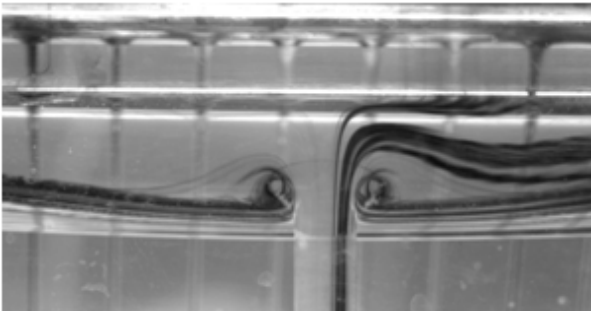
Figure 17: Influence of Reynolds number in the inlet pipe on vortex formation in the manifold for PVOH solution at \mu=110 mPa·s highlighted with tracers.
