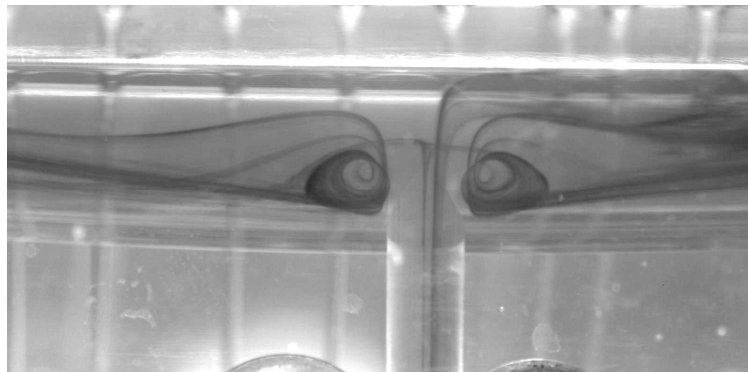
Figure 12 : An example of flow visualization with the tracer method.
