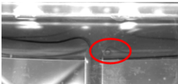
Figure 17: Influence of Reynolds number in the inlet pipe on vortex formation in the manifold for PVOH solution at \mu=110 mPa·s highlighted with tracers.
