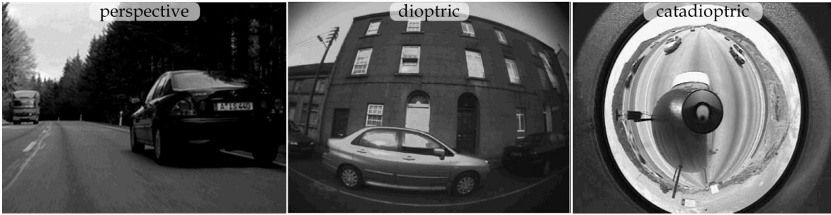
Figure 1.6: Perspective, dioptric 8 and catadioptric 9 images
