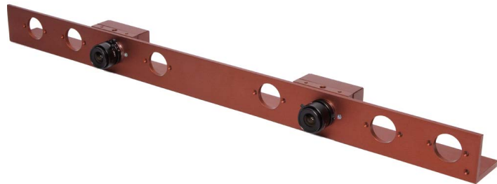
(b) Videre STH-MDCS-VARX composed of CMOS perspective cameras
