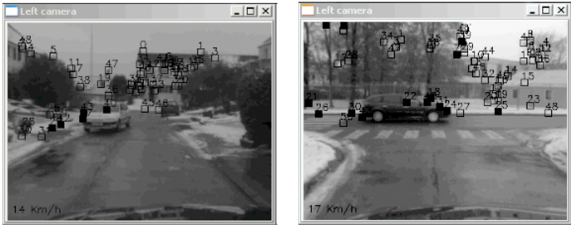
Figure 2.42: Outlier rejection of feature points lying on moving vehicles
