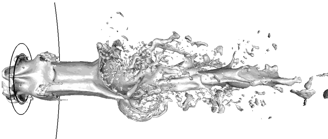
Figure 9: Interface location for the sheared annular liquid jet in Moreau and Desjardins [72]
