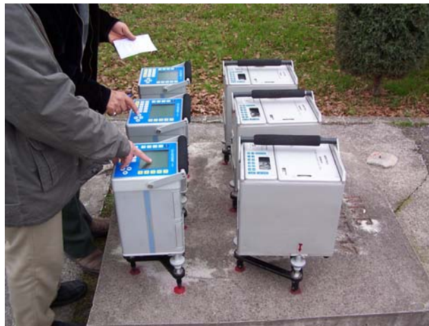
Photo. 3. Six Scintrex relative micro-gravimeters, 3 CG-5 (left) and 3 CG-3/M (right), used for calibration at NGCLI10 calibration line
