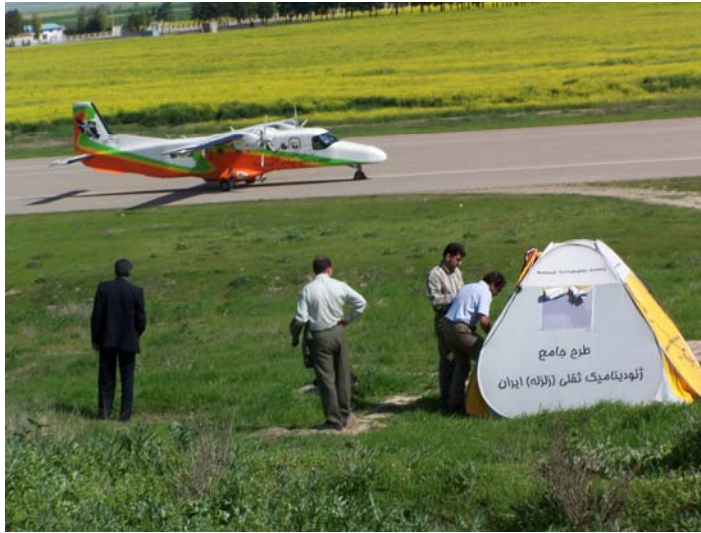
Photo. 2. Calibration of relative gravimeters (2004). Measurement at Kalaleh absolute gravity station (inside tent), belong to horizontal gravity calibration line of Iran (see Fig. 3.17, dashed red line). Transportation of gravimeters is done by NCC Dornier 228.
