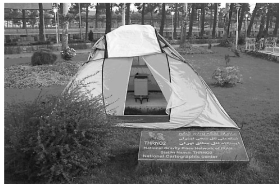
Fig. 2: Scintrex gravimeter at a gravity base station in Tehran
