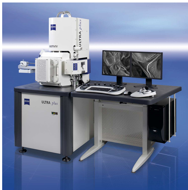
Figure III.7. FESEM Zeiss ultra plus (Carl Zeiss SMT-Nano Technology System Division)
