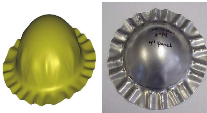
FIGURE 1.7 – Plissement de flan [Abderrabbo et al. 2005]
