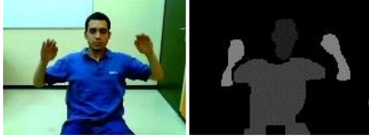
Figure 2-18: Segmenting regions from input image. The images are respectively: the captured image and the image segmented in three regions (arms, clothes and head).
