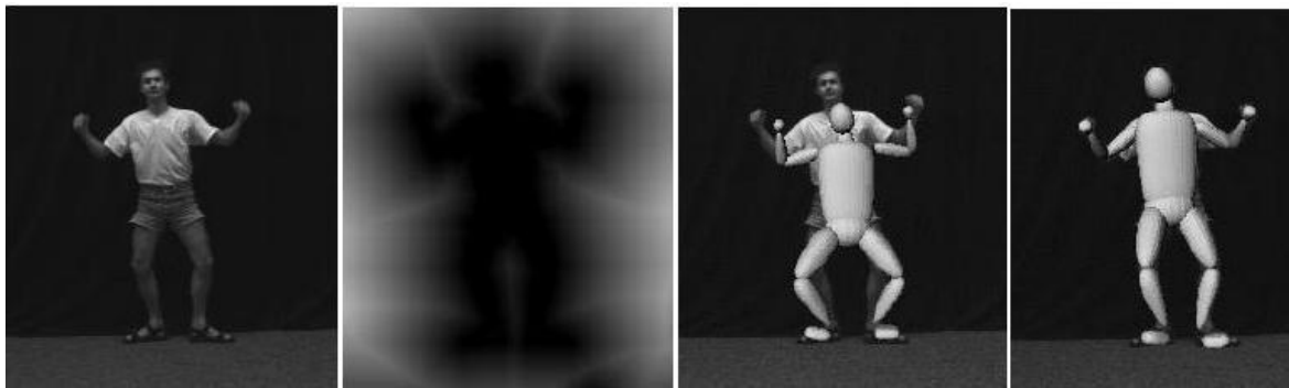
Figure 2-9: Generative Top Down estimation: 1) Input image, 2) Image feature, 3) Model projected in a candidate pose, 4) Estimation of model parameters by matching model projection and input image features (Sminchisescu, et al., 2002).
