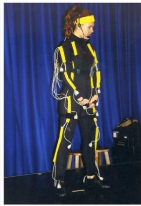
Figure 2-3 : A performer wearing a suit for magnetic motion capture (AMM, 2010)
