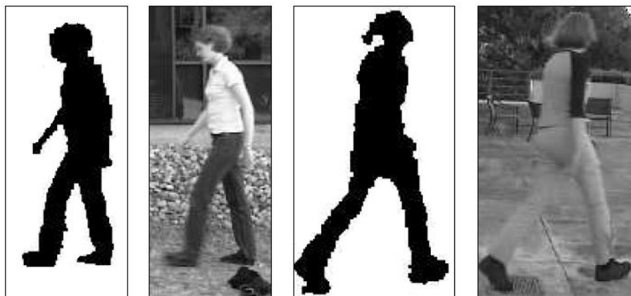
Figure 2-4 : Human silhouettes extracted using a background subtraction algorithm (Howe, 2006).
