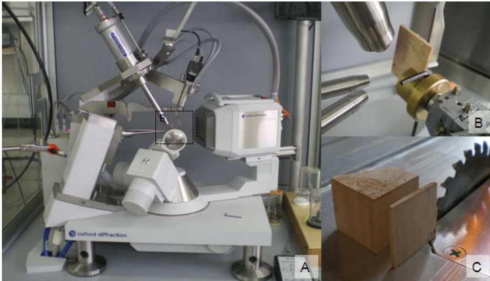
Figure 19 - X-ray diffractometer device with CuK \alpha radiation used for measuring XRD patterns (A), detail of the specimen holder (B) and the mini-circular machine used for cutting samples (C) (source: personal image)
