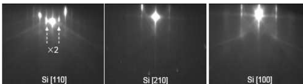
Figure III. 9 RHEED patterns of Si surface covered by 1/2 ML Sr, which lead to a \times 2 reconstruction along [110] direction.
