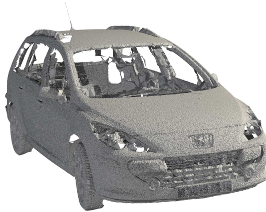
Figure 2.1: A Peugeot car acquired by a range laser scanner (acquisition made by Délégation Générale de l'Armement).
