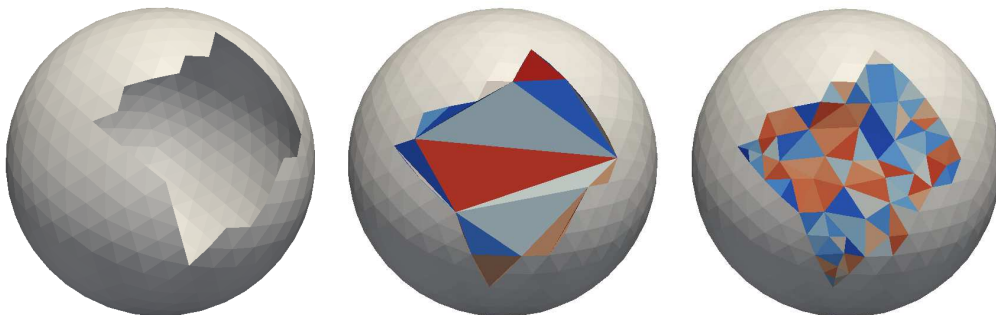
Figure 5.1: Initial hole (left), initial patch (middle) and refined patch (right).
