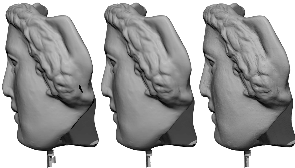
Figure 5.8: Mask: coarse scale mesh (left), coarse scale mesh with filled holes (middle), fine scale mesh with filled holes (right) . Here the base hole patch is removed.
