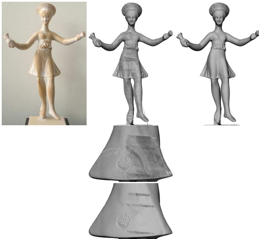
Figure 4.9: Merging of the Dancer With Crotales. From left to right: picture, without merging, with merging, an example of merging failure taken from the back of the object (top: unmerged, bottom merged)
