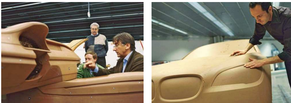
Figure 1.3 – Designer checking the physical form of a sculpture clay model. Images from BMW.
